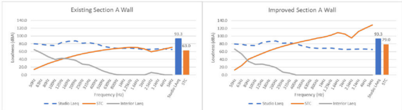
Figure 2. Existing Section A wall transmission loss on the left and the same wall with improvements on the right.
